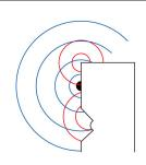
This diagram illustrates how energy from the tweeter (blue) is diffracted from cabinet edges and a nearby driver cavity (red).
