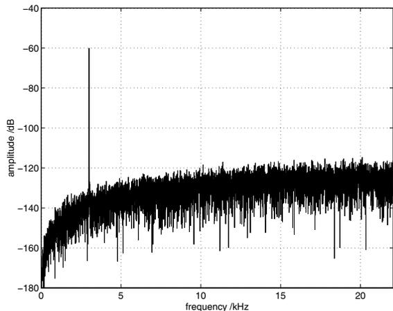
Figure 5: Quantised and noise shaped,  $H(z) = z^{-1}$ .
