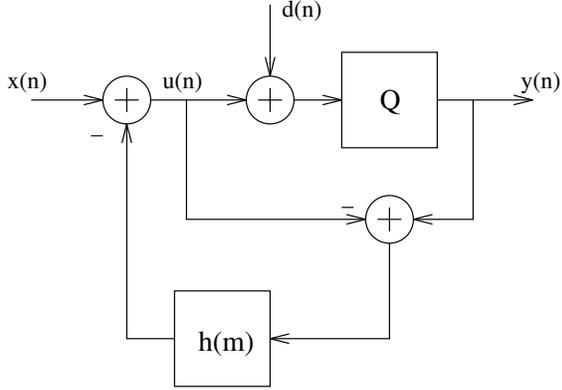
Figure 2: Noise-shaped Quantiser
