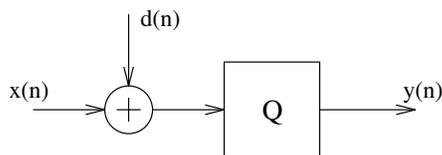
Figure 1: Simple dithered quantiser
