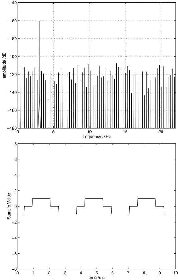
Figure 3: Undithered Quantiser
