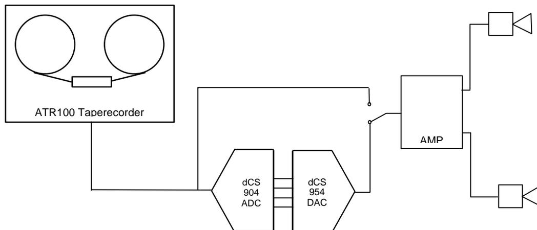
Figure 1 – High Sample Rate Demonstration setup
